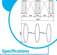
Clear Walkway-adjustable: 500-550 mm : Motorized : Wooden Top Cover **Top Cover Front Cover** : 304 Grade SS Wing Housing : 304 Grade SS Indicators : LED on one side
